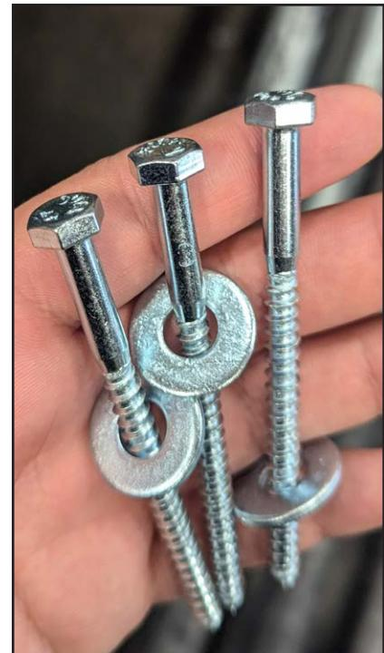
Depending on the type of spa, a piece of wood is placed on the side panels of the spa to protect it in shipping. The wooden supports are installed with several  $7/16$ " (11mm) bolts, once the spa is in its final resting place, remove these with an 11mm socket.
