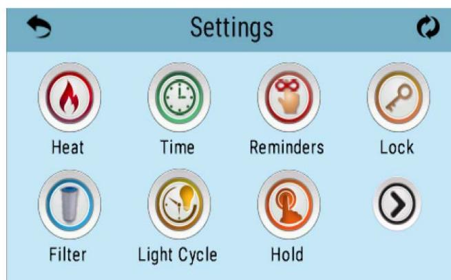
The settings screen is where all programming and certain spa operations are controlled. Each icon leads to a sub menu that can toggle specific parameters that fall under the mentioned option.
